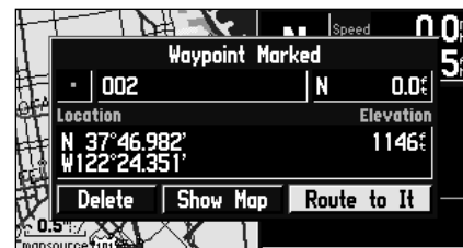
An example of a “button”—the ‘Route to It’ button on the Waypoint Marked Page.
